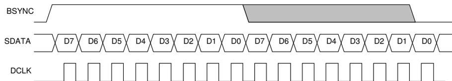
Figure 4: BSYNC Signal - two byte transfer.
