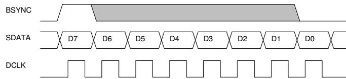
Figure 3: BSYNC Signal - one byte transfer.
